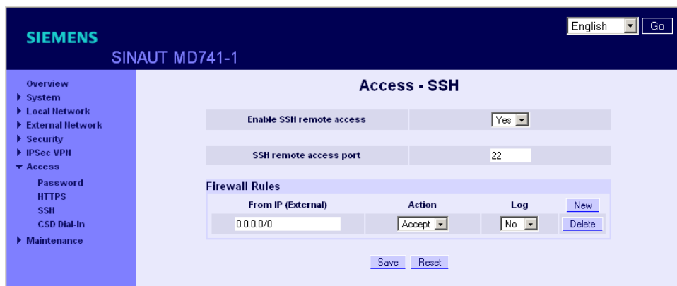
Figure 8-2 Access >SSH remote access
